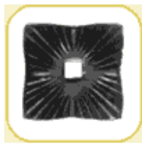
Square shaped and patterned base plate 75x75x5mm with 13mm hole to suit 12x12mm bar upright
